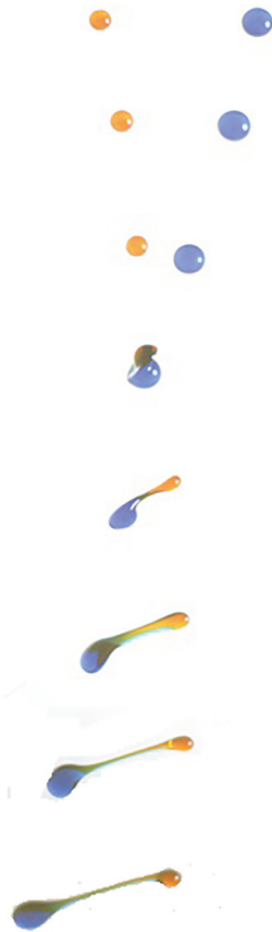
Fig. 6. Grazing collision of unequal-size colored oil drops with We \sim 20 ; the orange drop has diameter \sim 3 mm and the blue drop has diameter \sim 5 mm. Also, see the videos available as supplementary material (Ref. 34).
