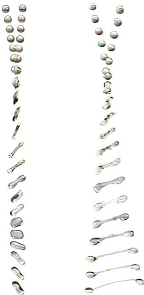
Fig. 4. Left: Shape evolution of head-on collision ( b=0 ) of equal size oil drops \sim 6 mm in diameter with We \sim 10 (see Tables II and III). Right: same as the left panel but for a grazing collision ( b > 0 ) with We \sim 100 . Also, see videos available as supplementary material (Ref. 34).
