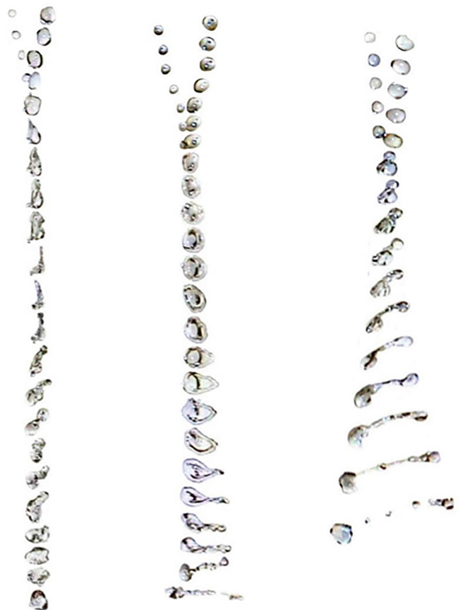
Fig. 7. Shape evolution for water-drop collisions (see Tables II and III) for unequal size drops \sim 4 and 7 mm in diameter for various impact parameters: (left) We \sim 15 ; (center) We \sim 80 ; (right) We \sim 250 . Also, see the videos available as supplementary material (Ref. 34).
