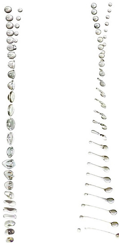
Fig. 5. Oil drop collisions with unequal size drops \sim 4 and 6 mm in diameter with We \sim 20 (see Tables II and III). Left: head-on collision ( b=0 ); Right: grazing collisions ( b > 0 ). Also, see videos available as supplementary material (Ref. 34).
