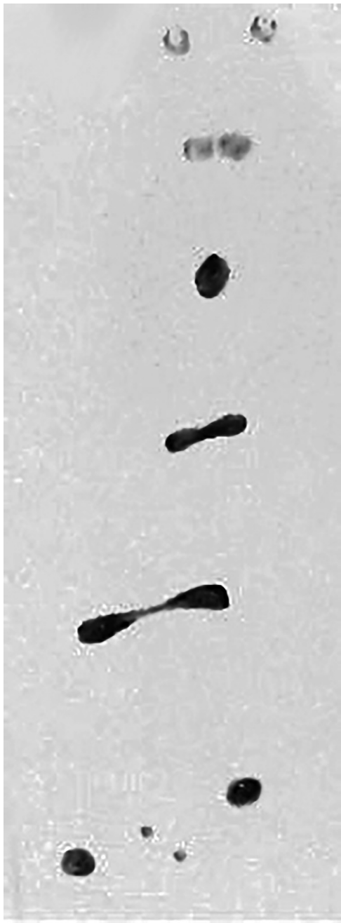
Fig. 10. Near head-on collision of charged oil drops, diameter \sim 6 \mu\text{m} ( V = 35 kV). Also, see the videos available as supplementary material (Ref. 34).
