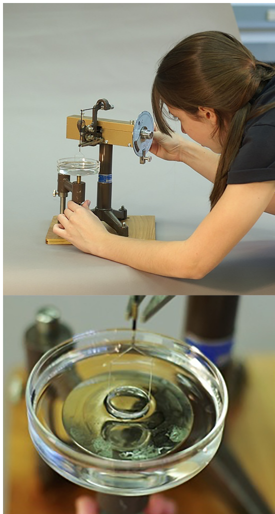
Fig. 3. Top: A student measuring force to determine surface tension of a liquid. Bottom: Close up of ring apparatus used to measure surface tension of a fluid.
